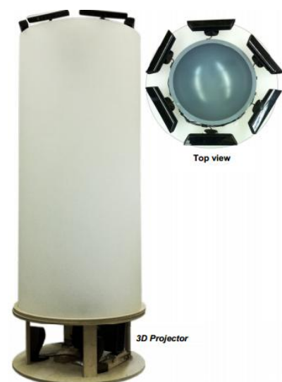
Figure 3: The TeleHuman hardware- a cylindrical display surface with 6 Kinects and a 3D projector in base
